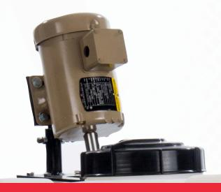
The agitation is what keeps your product in suspension throughout the injection process. The **mechanical agitation** can be driven by 3PH, 1PH,or 12 volt motors. The prop and shaft are made of 316 stainless steel for maximum durability. Mechanical agitation is recommended for products that need vigorous mixing to stay in solution. Air agitation (pictured on the next page) is also available. Air agitation is used for products that do not need vigorous mixing to stay in solution.
