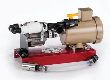
The **Inject-O-Meter Air Agitation** is comprised of a high volume, low pressure air pump that delivers constant air to the bottom of the chemical tank through a sparger nozzle.
