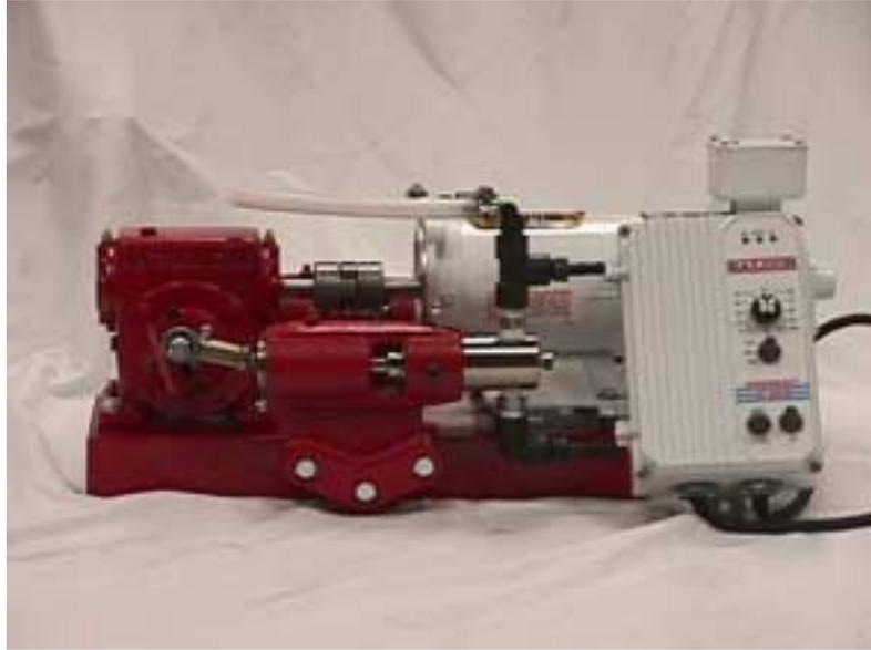
A simple and economical way to change the output of the injection pump without having to manually adjust the stroke length.
